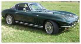
This was the last Corvette that Dick Guldstrand built. In 2009 Victoria Hearst discussed having an older body-style Corvette built on a newer frame. A 1965 was placed on a C4 frame from Newman Car Creations and was fitted with an LS1 engine. Guldstrand massaged the 346 ci. V8 to 400 hp and installed a four-speed automatic transmission since Hearst couldn't drive a stick. A good bit of fabrication and custom work went into this build.
